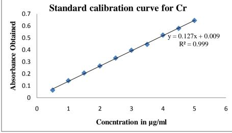
Figure 1: Standard Calibration Curve for Estimation of Cr in Samples.
