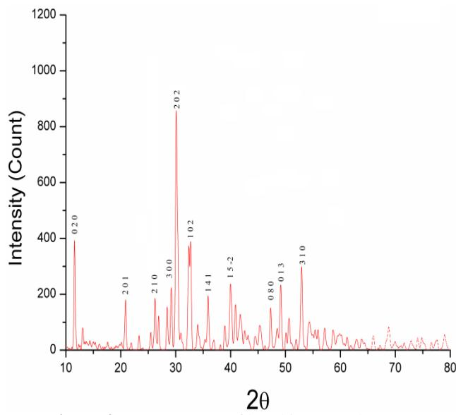
**Figure 3:** XRD pattern of brushite crystals
