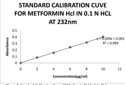
Figure 2: Standard Calibration Curve Of Metformin Hcl In 0.1n Hcl
