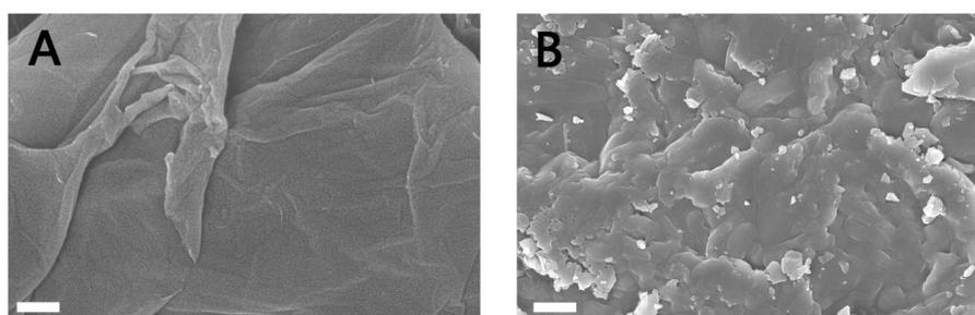
**Figure 4.** SEM images of lyophilized GO (A) and GO-CAPT (B). Scale bar:  $1\ \mu\text{m}$ .
