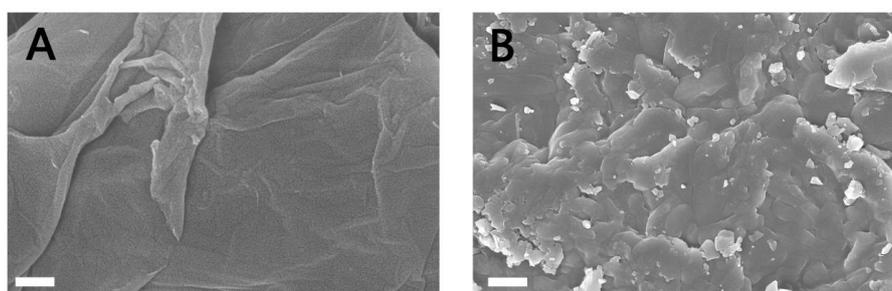
**Figure 4.** SEM images of lyophilized GO (A) and GO-CAPT (B). Scale bar:  $1\ \mu\text{m}$ .
