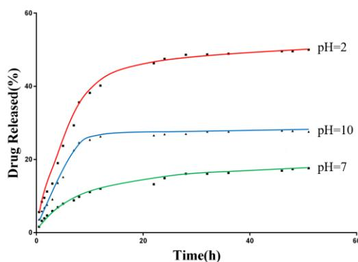
**Figure 6.** Yields of drug released from freeze-dried carrier at different pH values.
