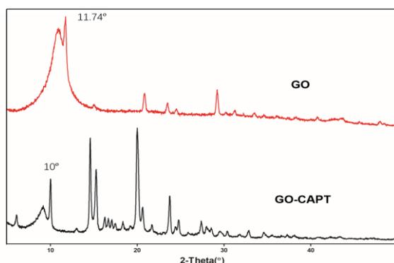
**Figure 2.** XRD spectra of GO and GO-CAPT.
