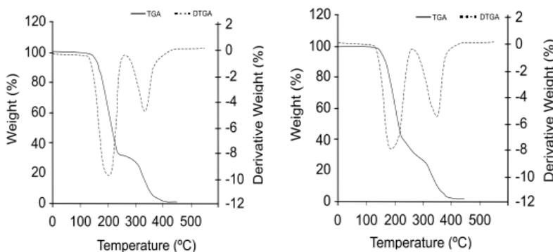
**Fig. 10. TGA Thermogram of PS - PCL Blend<sup>28</sup>**
