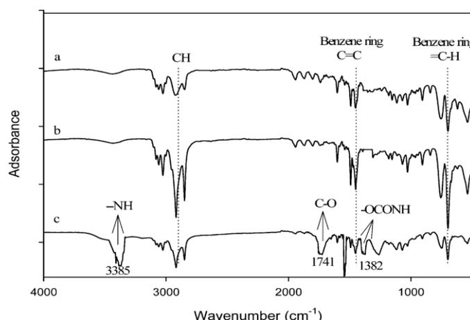
**Fig. 7. FTIR Spectra of PS - PU blend (c)<sup>11</sup>**
