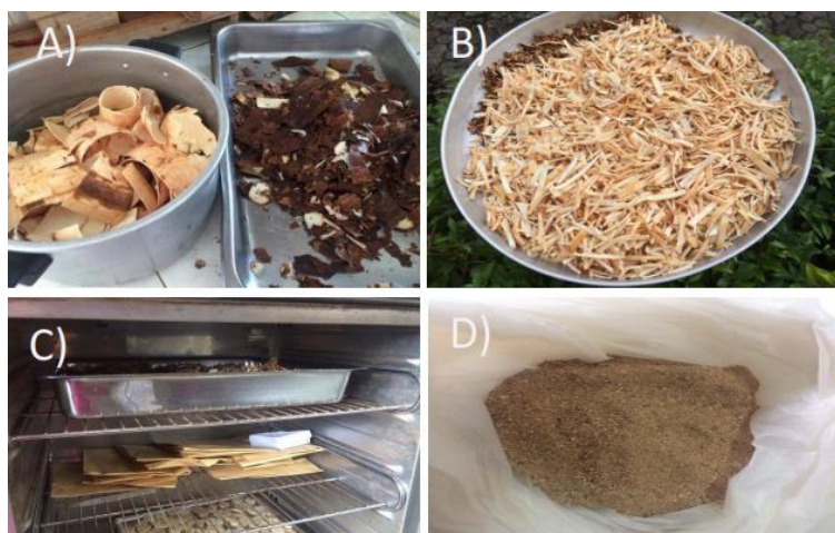
Fig 2. Cassava peels samples were prepared by (A) washing, (B) cutting, (C) drying, and (D) grinding processes 20
