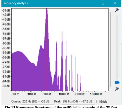
Fig.13 Frequency Spectrum of the artificial harmonic of the 7<sup>th</sup> fret
