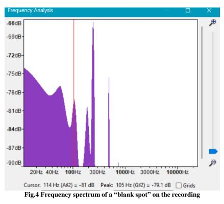
We observe a peak at 105 Hz even when no string is being plucked. This indicates that the peak at 105 Hz is produced due to the background noise that the recorder has recorded.
