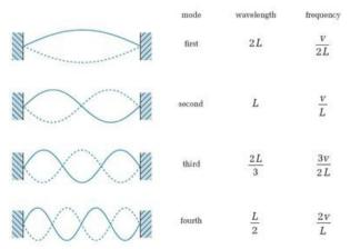
Fig.2 The first four normal modes of vibration of a string are fixed at each end. The solid and dashed lines indicate the positions of the string at opposite phase positions in the cycle.
