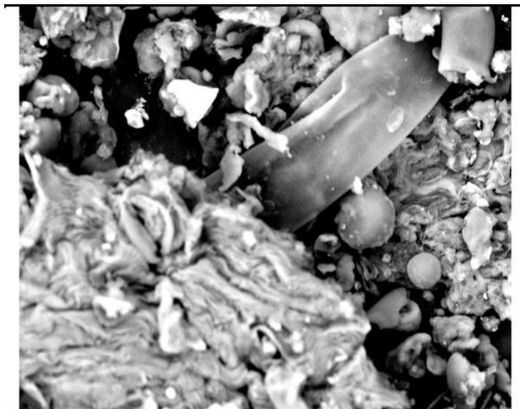
Figure 10c. SEM micrograph of Sample A (Bitter leaf extract)–showing mixed flaky and granular fragments at higher magnification.
