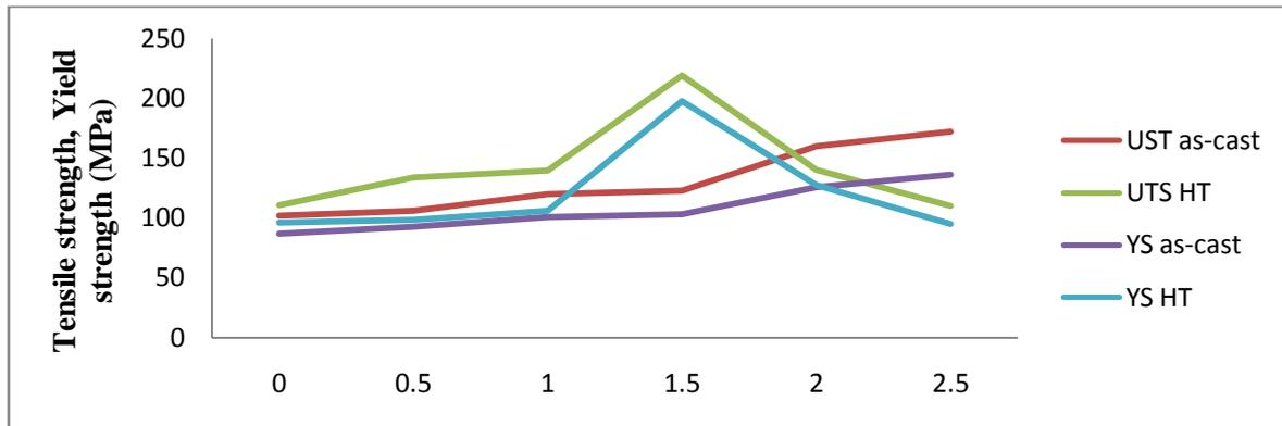
**Fig. 1. Tensile properties versus Mg content**
