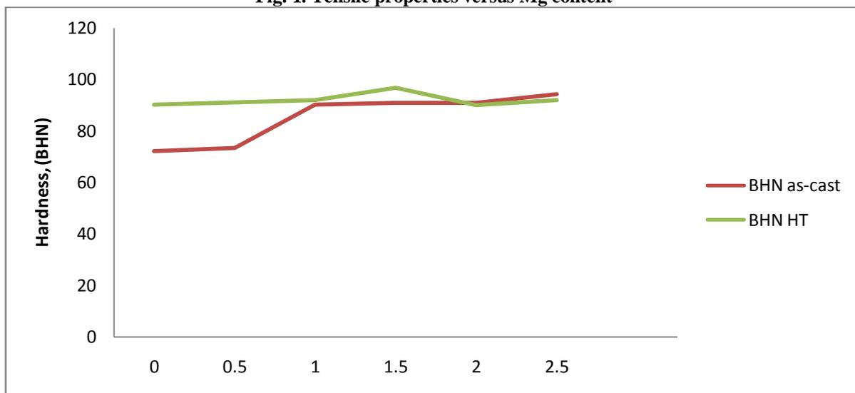
**Figure 2. Hardness versus magnesium content**
