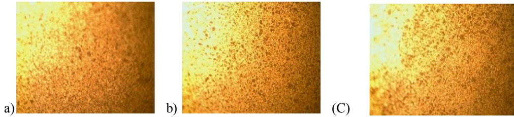
Fig. 6 Microstructures of medium carbon steel austenitized at 900°C, quenched and tempered at 350°C a) (mineral oil; b) neem oil; c) watermelon oil x200.
