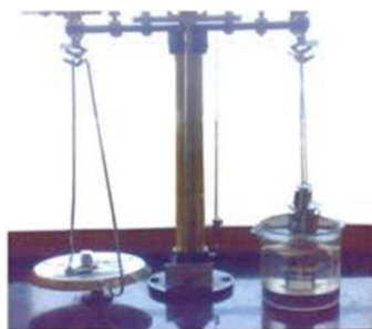
Figure 1: Modified analytical balance for mucoadhesive strength measurement
