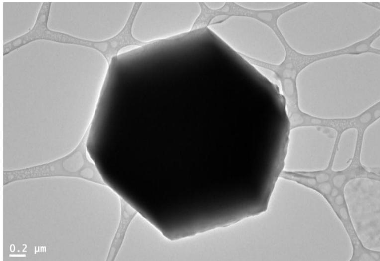
**Figure 1:** Transmision electron microscope (TEM) images of ZnO nanoparticles sample. Images was captured in 0.2 micrometer scale bar.
