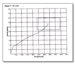
Fig. 9: Mean Tenacity vs E Line Graph of Dyed Corn Fiber at  $90^{\circ}$ C
