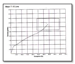
Fig. 8: Mean Tenacity vs E Line Graph of Undyed Corn Fiber
