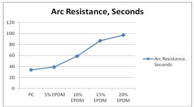
Figure 2 Arc Resistance of PC and PC-EPDM blends
