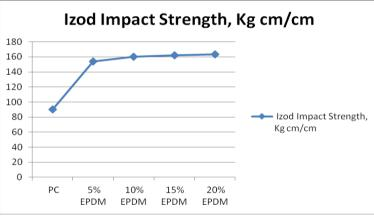
Figure 1 Impact Strength of PC and PC-EPDM blends
