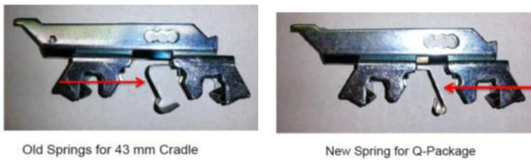
(A) (B) Fig.7. Old springs (A) and new spring (B).
