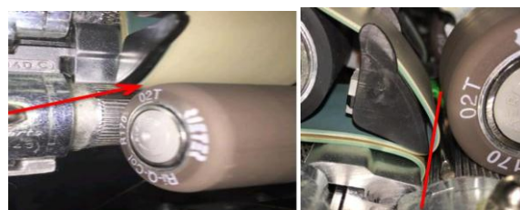
(A) (B) Fig.8. Correct setting of nose bar and cradle.
