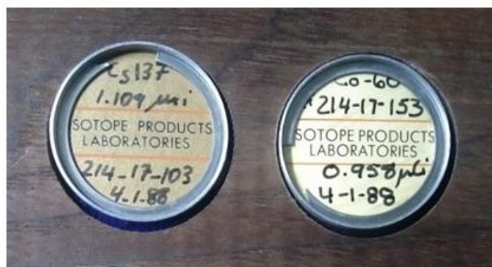
Figure no 1: Gamma radioactive point sources ^{137}\text{Cs} & ^{60}\text{Co}
