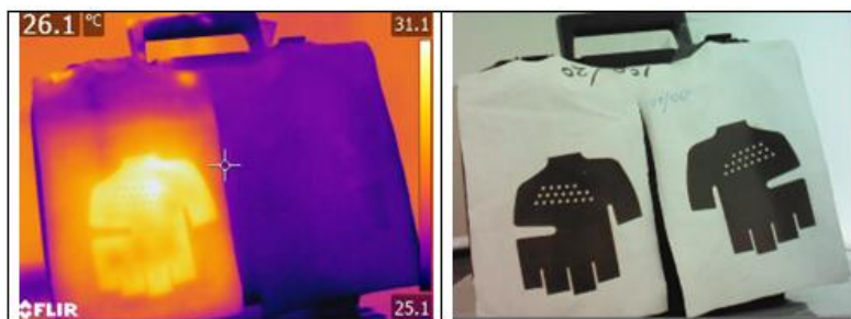
Figure 5: 5% w/w tourmaline powder infused fabric shows increase of temperature up to 26.1°C compared to same fabric with same design without the addition of tourmaline powder (after 10 min of exposure to radiation).
