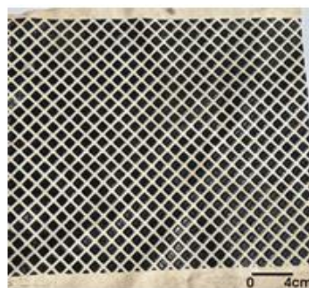
Figure 2: Tourmaline infused cotton fabric having alternating hump and valley texture (0.5-1 mm)
