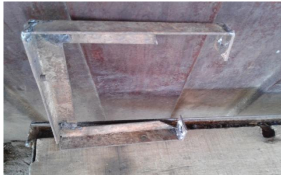
Figure. 3: Alternator Frame (3-angle bar steel)
