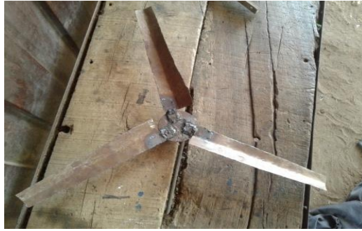
Figure 2: constructed Turbine (3-dimensional blade)
