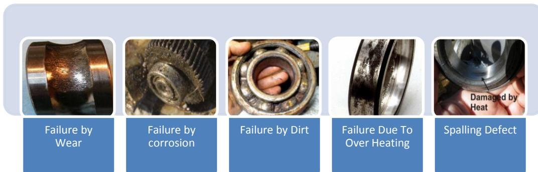
**Figure 4 Types of Bearing Failure**
