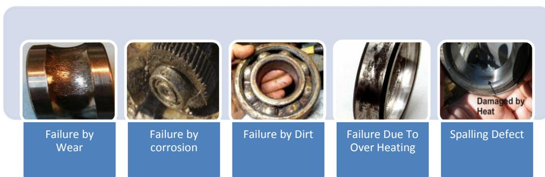
**Figure 4 Types of Bearing Failure**
