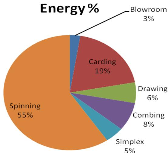
**Figure 1. Power consumption of various departments in spinning mill.**
