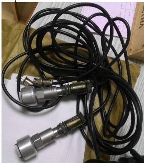
**Figure 5 Accelerometer**
