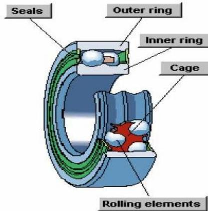
Figure 2 Components of bearing
