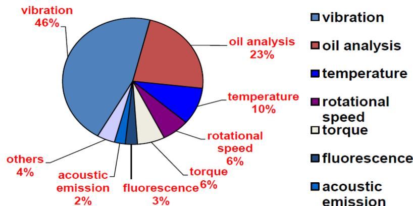
Figure 3 Causes of bearing failure
