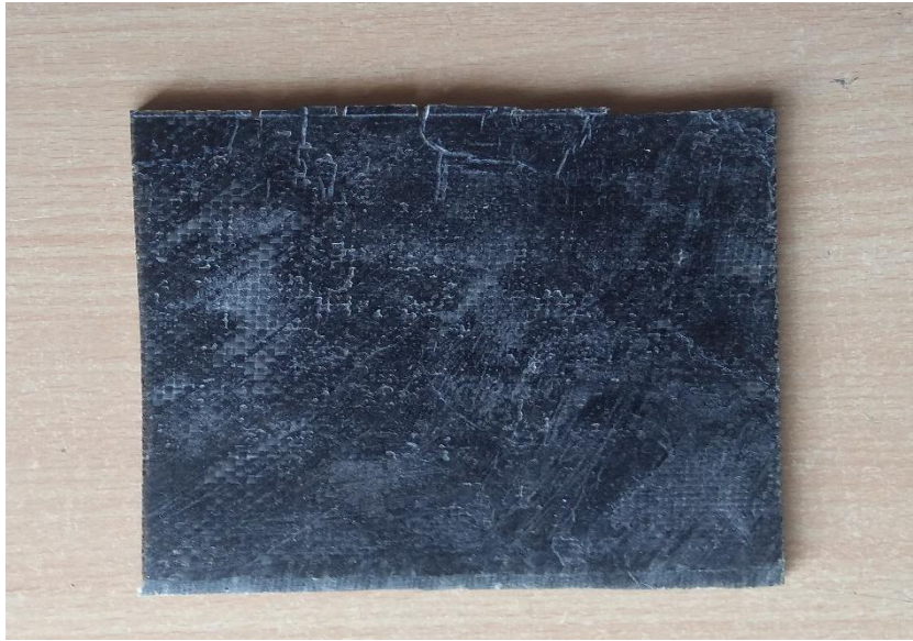
Fig. 1 Fabricated Hybrid Laminate
