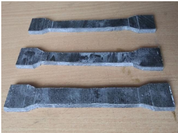
Fig. 2&3 Tensile and impact test samples
