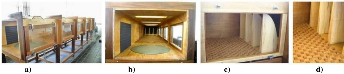
Figure 3. Side [a] and frontal [b] views of the wind tunnel. Obstacles acting as turbulence generators [c] and rough surface [d] of the FAU / UFRJ wind tunnel.
