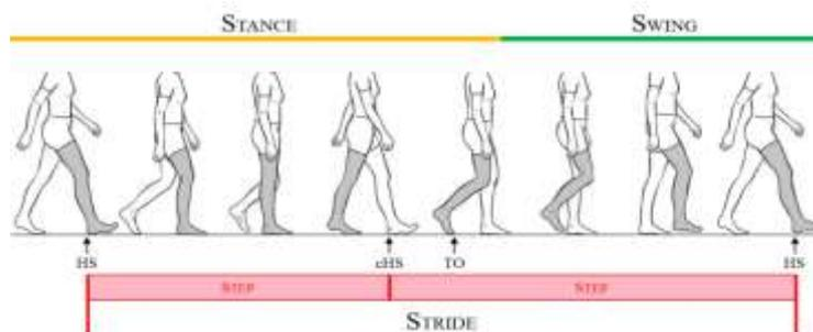
**Figure 2:** Subdivision of gait cycle on the basis of foot contact data (HS, heel strike; cHS, contralateral heel strike; TO, toe off).
