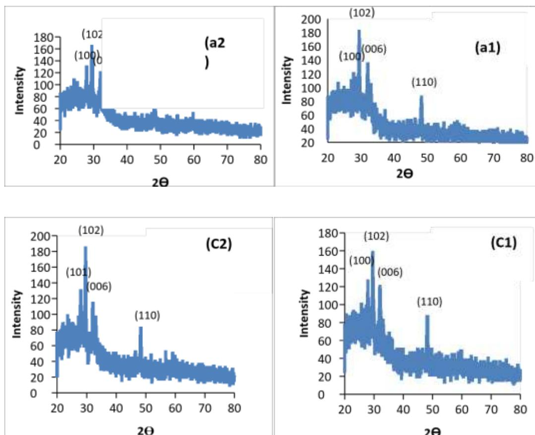
**Fig (1).** XRD pattern of CuS thin films (CuCl<sub>2</sub>.2H<sub>2</sub>O + TU) for different molar concentration, a1, b1 for as deposited films and a2, b2for annealed films (T= 150 °c for 1 h.).
