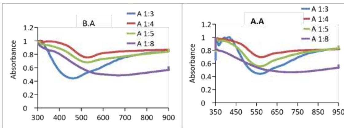
Fig.5.shows Absorbance transmission spectra of the CuS films; as deposited and(A.A) annealed films with different molar ratio.
