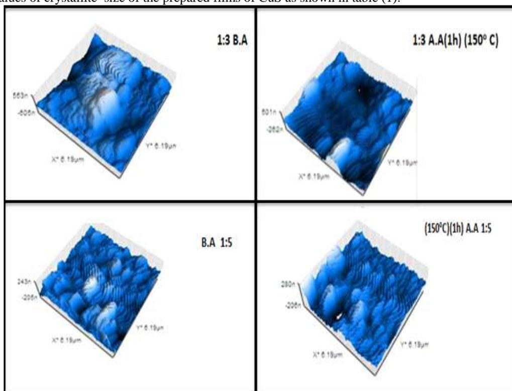
**Fig . 3.** Results of (AFM) for CuS thin films; as deposited and annealed films for molar concentration ratio (1:3 and 1:5)
