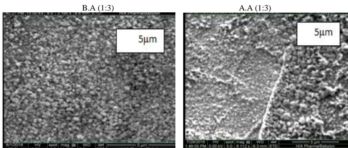
**Fig .2.** Shows images of (SEM) for CuS thin films; as deposited and annealed films with molar concentration ratio (1:3).
