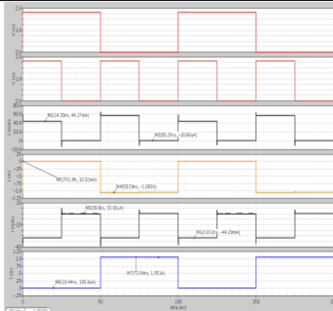
Fig. 7- Current at the source and substrate terminals of the pMOS and nMOS of input stages
