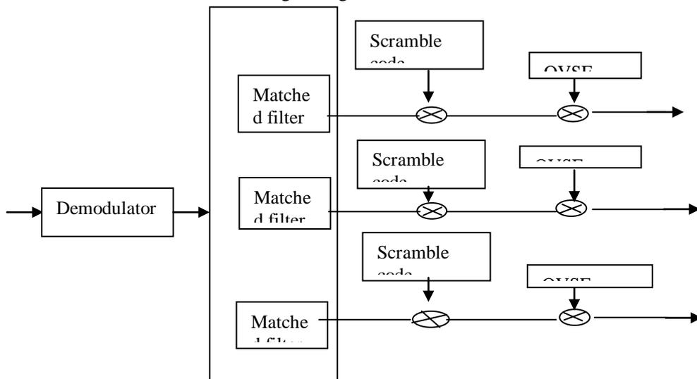
Figure 5: Receiver Module
