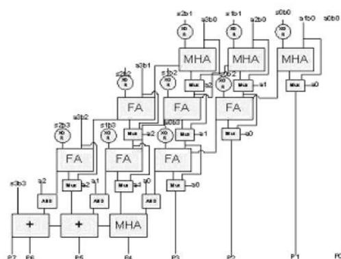
Figure 8. A 4x4 multiplier structure.
