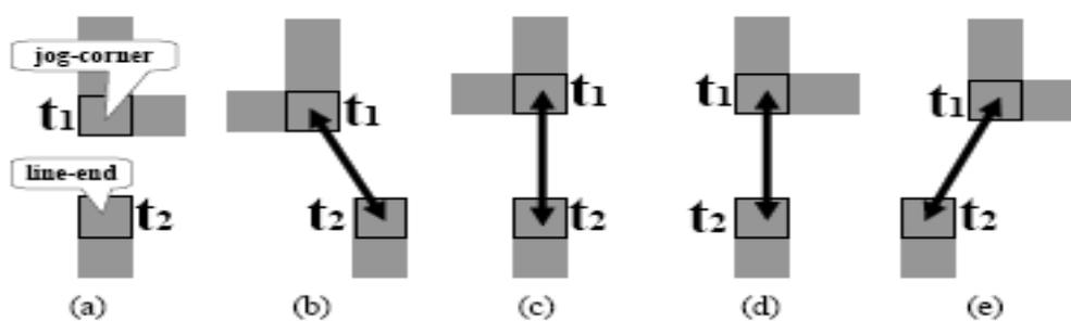
Fig. 2. Characterization for  $t_1$  jog-corner and  $t_2$  line-end is shown where (b), (c), (d), and (e) are the cases with the same distance. Thus, the mean EPE will characterize this interaction between  $t_1$  and  $t_2$  at this distance.
