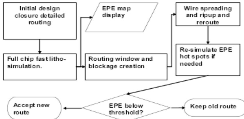
Fig. 1. EPE based construct-by-correction in the model-based method [4].
