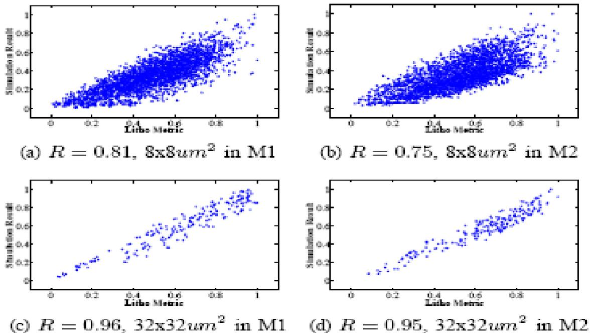
Fig. 3. The litho-metric shows higher fidelity to post-OPC printability in large scale.
