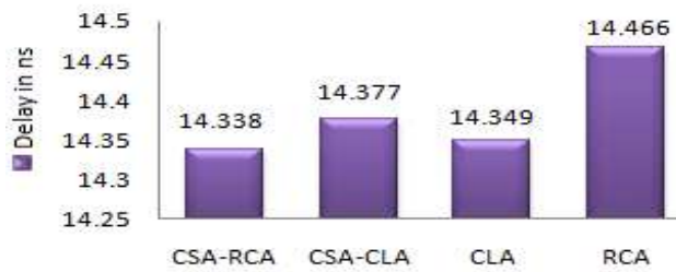
Figure 9. Delay comparison among different adders for addition of four eight bit numbers
