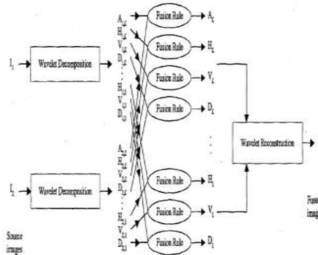
Fig.1 Wavelet based Image Fusion Procedure
