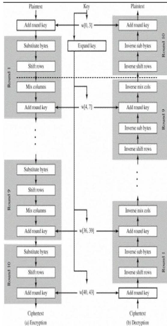
Fig.1. Block diagram of AES Algorithm
