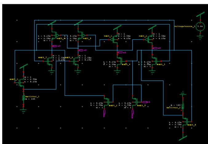
Figure 13: BQCCM10T cell design
