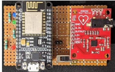
Figure 1: Hardware setup for ECG Signal Capture
