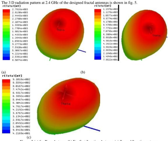
Figure 5 (a) for Base Antenna (b) For first Iterative Antenna (c) Second Iterative antenna
