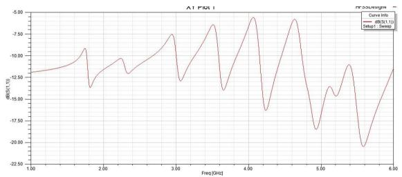
Figure 3 S<sub>11</sub> Vs frequency curve for first iterative modified fractal microstrip patch antenna
