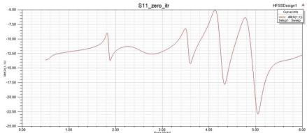
Figure . 2 S<sub>11</sub> Vs frequency curve for base form of the modified fractal antenna
