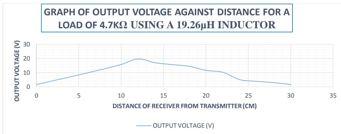
**Fig. 9:** Graph of Output Voltage against Distance for a Load of 4.7KΩ while using a 19.26μH inductor.
