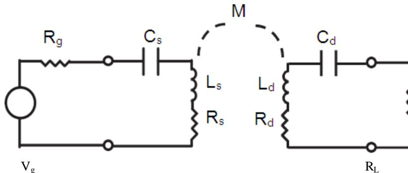
Fig. 2: Equivalent circuit for the coupled resonator system
