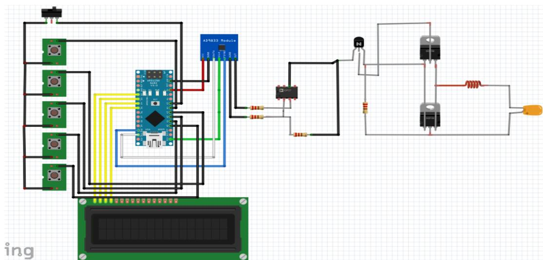
Fig. 3.2: Circuit Diagram of the Complete Transmitter System
