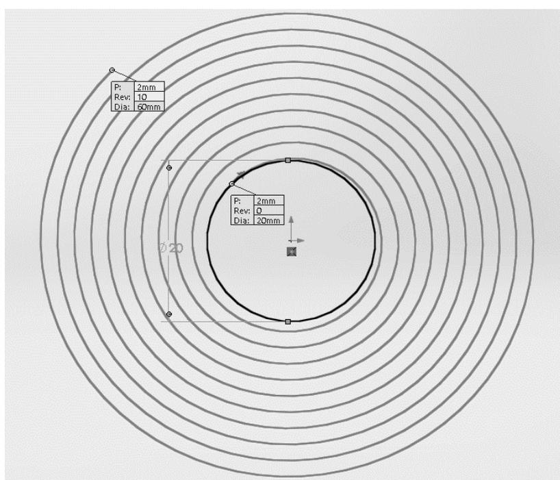
Fig. 3.3: SOLIDWORKS Design of Flat Spiral Coil
