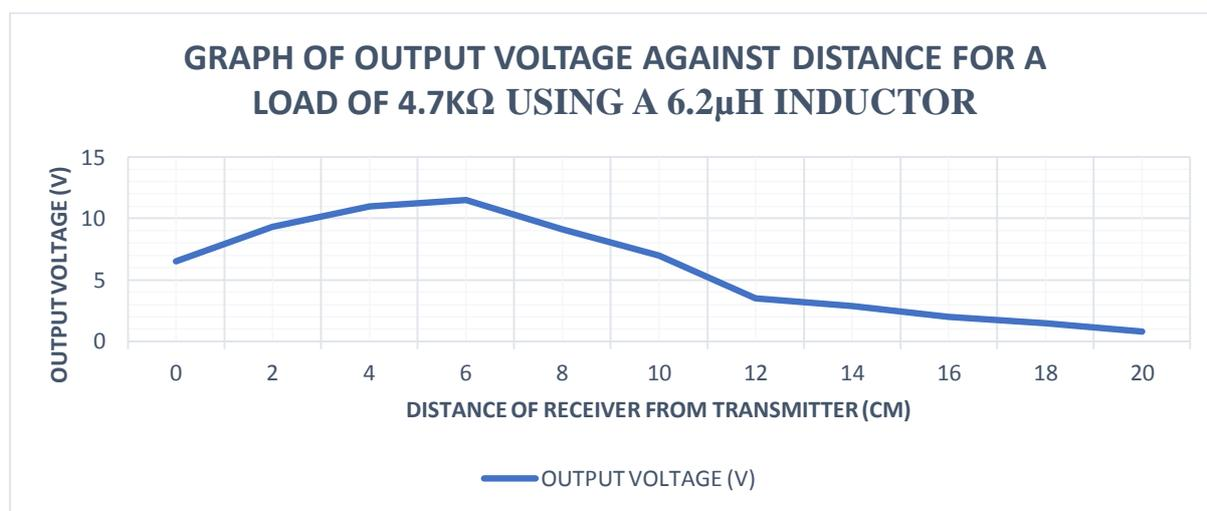
**Fig. 8:** Graph of Output Voltage against Distance for a Load of 4.7KΩ while using a 6.2μH inductor.
