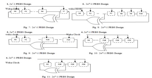
**Description:** Fig. 7 shows PRBS-7 Sequence with tapping points 7 and 6 and sequence length is  $2^7$ -1 times the repeat sequences generated. Fig1.6 PRBS-10 Sequence with tapping points 10 and 7 and sequence lengths is  $2^{10}$ -1 times repeat the sequence.similarly other PRBS Sequences 15,23,31,48,52,63 with repeated pattern sequence lengths are  $2^{15}$ -1,223-1, $2^{31}$ -1, $2^{48}$ -1, $2^{52}$ -1, $2^{63}$ -1.
