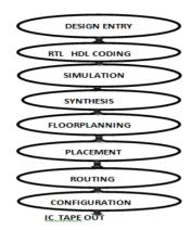
Fig. 12: VLSI IC-EDA Software Design Flow Chart
