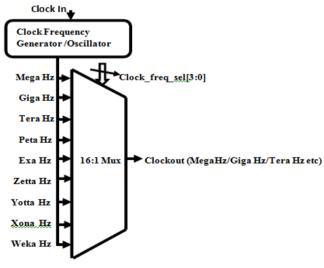
Fig.1: Multi Clock Frequency Generator
