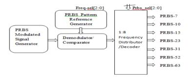
Fig.4: Multichannel PRBS Receiver Architecture
