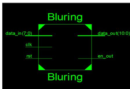
Fig.3 (b). RTL Top module Schematic of Image smoothing (thin blurring) Unit
