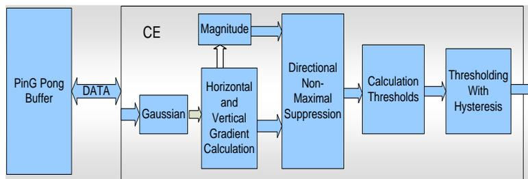
Fig. 2: Block diagram of the compute engine.
