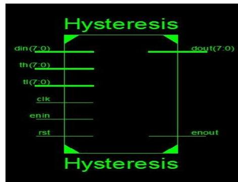
Fig.5 (b) RTL Top module Schematic of Hysteresis Unit.
