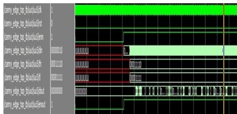
Fig.5(c).Simulation Results of Hysteresis Unit.
