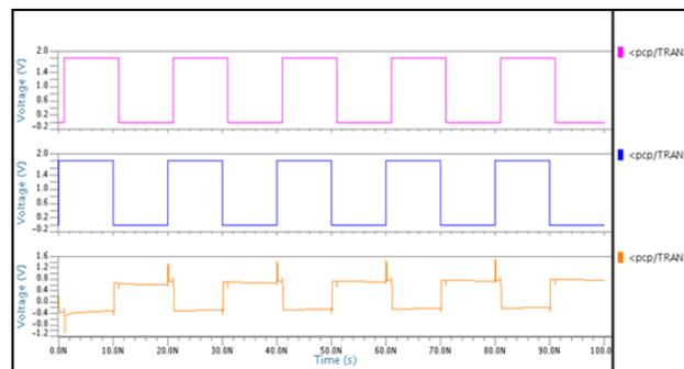
Fig. 4 Waveform of Charge Pump
