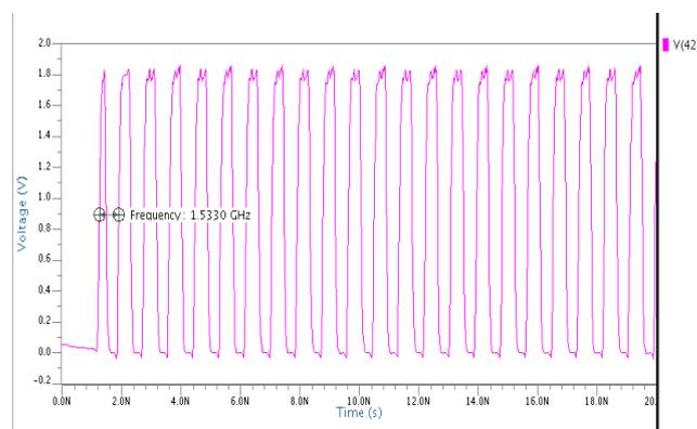
Fig. 10 Simulation result of VCO at 90mV input voltage
