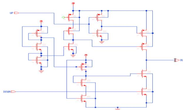
Fig. 3 CMOS circuit of Charge Pump [4]
