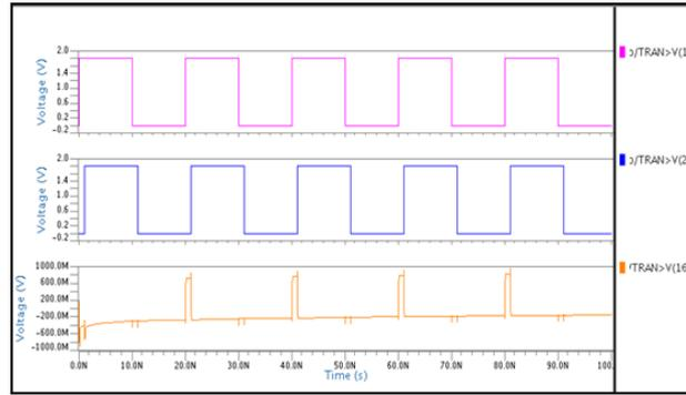
Fig. 5 Waveform of Charge Pump with PFD
