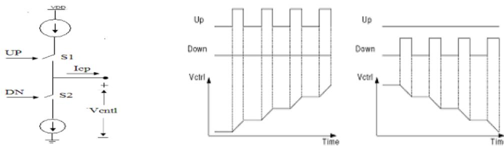
Fig 2 Basic block diagram of Charge Pump with Ideal Behavior [1]
