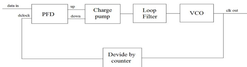
Fig 1 A Basic Block Diagram of Phase Locked Loop [1]
