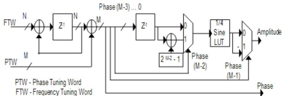
Fig.2: Direct Digital Frequency Synthesizer
