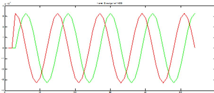
Fig. 6: Simulated Output of DDS
