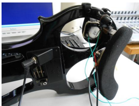
Fig.1. Hardware Setup of Feedback actuators to the electronic violin
