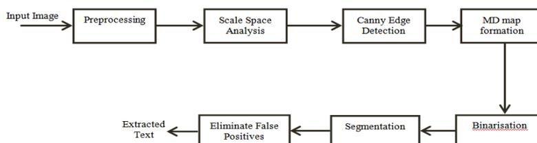
Fig. 1: Block diagram of the proposed method
