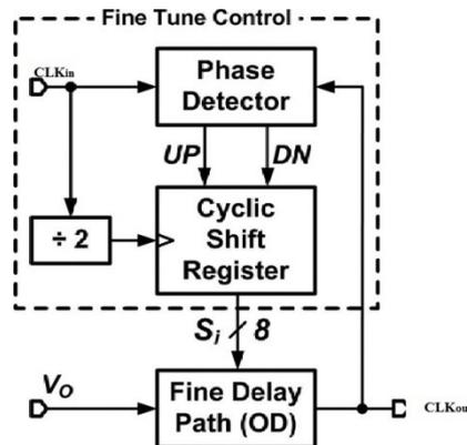
fig.3 Block diagram for fine tune control
