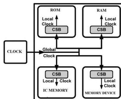
fig. 1 Clock distribution in an SoC
