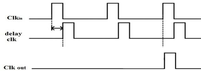
fig.4 synchronization of two clocks
