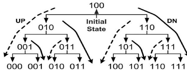
fig.5. SAR algorithm
