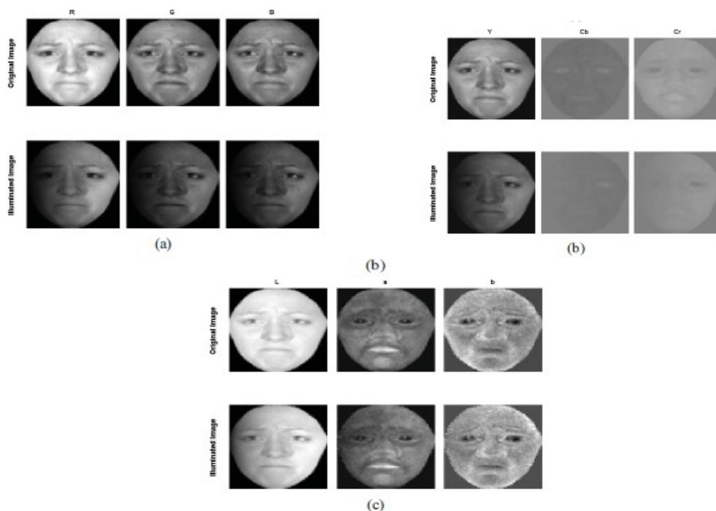
Fig. 11. Facial expression images in (a) RGB, (b) YCbCr, (c) CIE Lab, and color spaces. Top row: original image.
