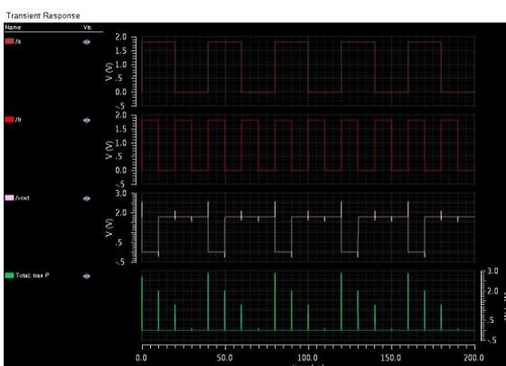
Fig.(h)NAND waveform without transistor sizing
