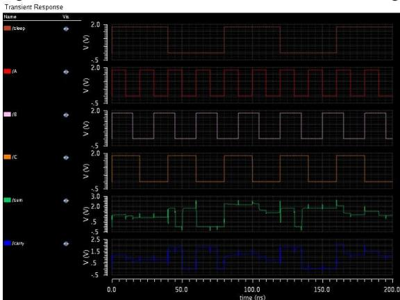
Fig.(u) 28T adder waveform with MTCMOS
