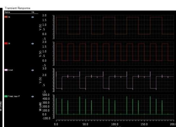
Fig.(i) NAND waveform with transistor sizing
