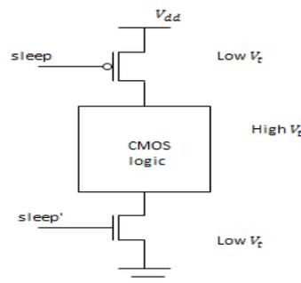
Fig.(f) MTCMOS circuit
