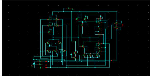
Fig.(e) Schematic View of 28T Adder Circuit
