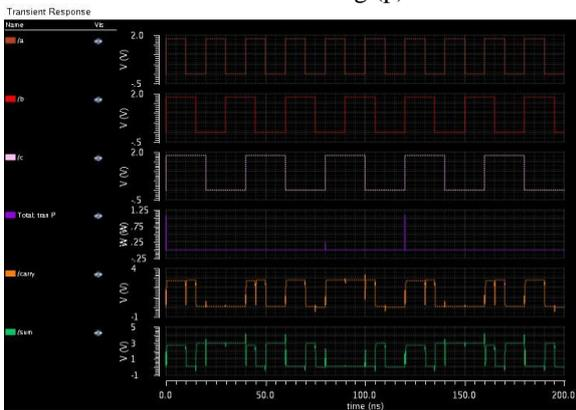
Fig.(q) 36T adder waveform with MTCMOS
