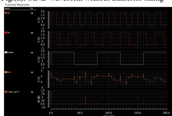
Fig.(j) NAND waveform with MTCMOS Technique
