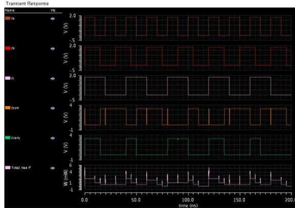
Fig.(p) 36T adder waveform with Transistor sizing
