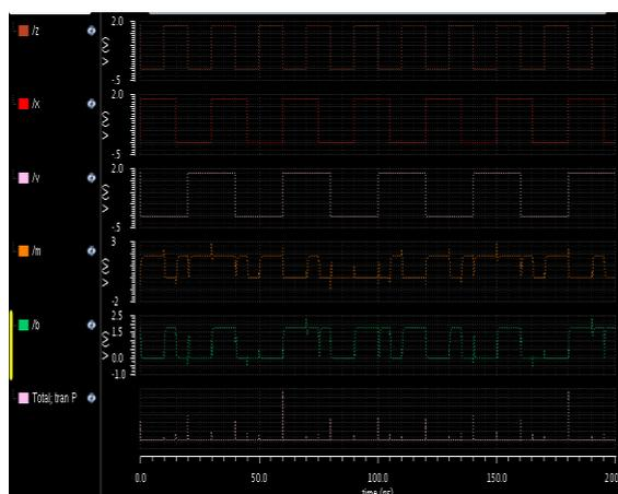
Fig.(n) 58-T adder waveform using MTCMOS
