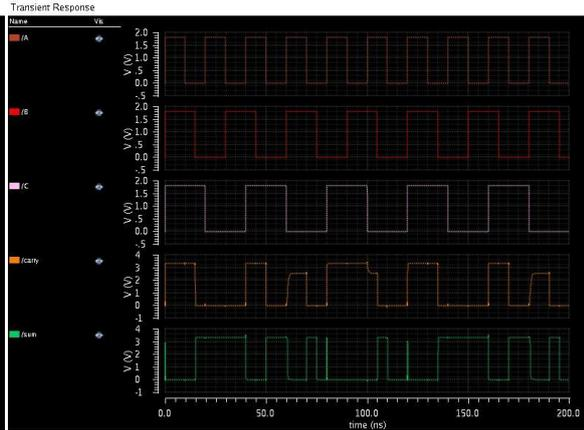
Fig.(t) 28T adder waveform with Transistor sizing
