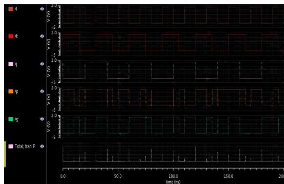
Fig.(l) 58-T adder waveform without transistor sizing
