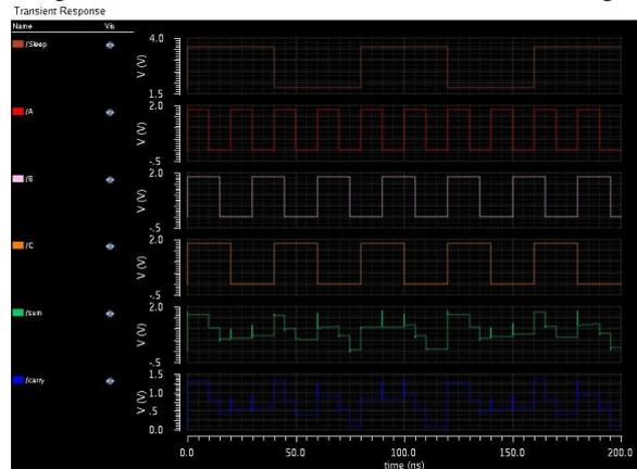
Fig.(v) 28T adder waveform with combined tech.
