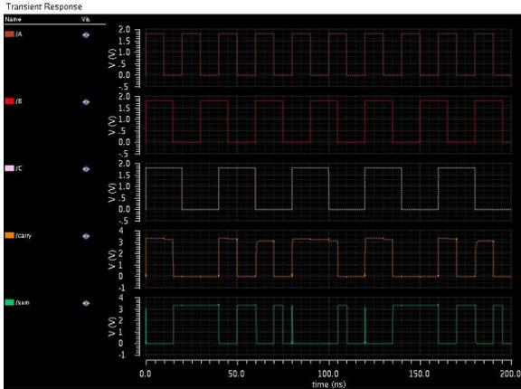
Fig.(s) 28T adder waveform without Transistor sizing
