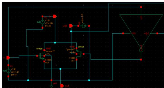
Fig.(w) Schematic of transmission gate
