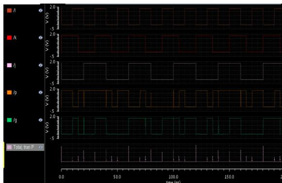
Fig.(m) 58-T adder waveform using transistor sizing
