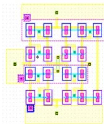
Fig.8: Layout of third generation current conveyor
