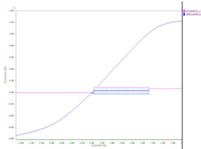
Fig.3: DC transfer characteristic of  $I_y$ ,  $I_x$  and  $I_{z+}$
