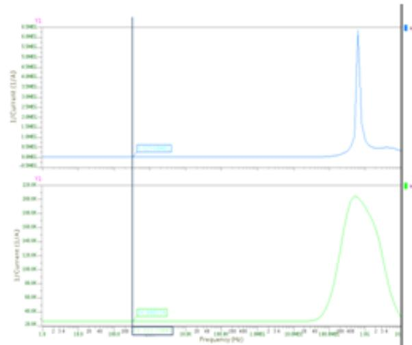
Fig.6: AC response of trans impedance  $R_x$ ,  $R_z$
