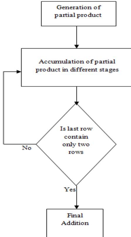
Fig. 2 Flowchart for designing a conventional wallace multiplier
