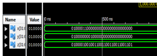
Figure 5: Simulation result of Radix-8 based floating point division
