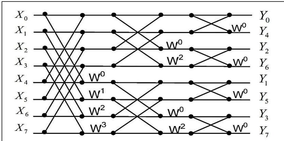
Figure 2: 8-Point Radix -2 DIT FFT Using Butterfly Structure
