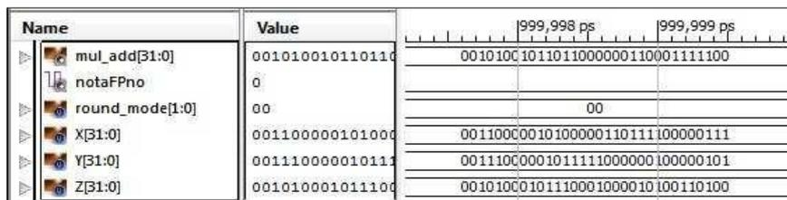
Figure 7 Timing Simulation waveform of Proposed FFPMA module
