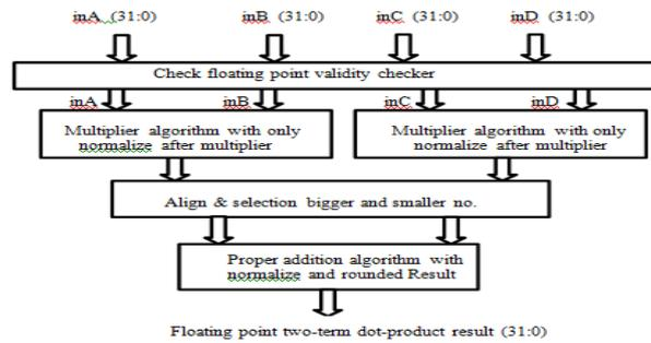
Figure 8 Flowchart of Proposed Fused floating point Two-term Dot Product (FFP2TDP) module
