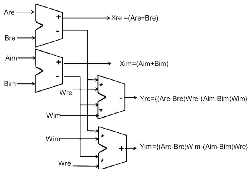
Figure 10 Proposed Fused Floating Point implementation of Radix 2 FFT butterfly structure
