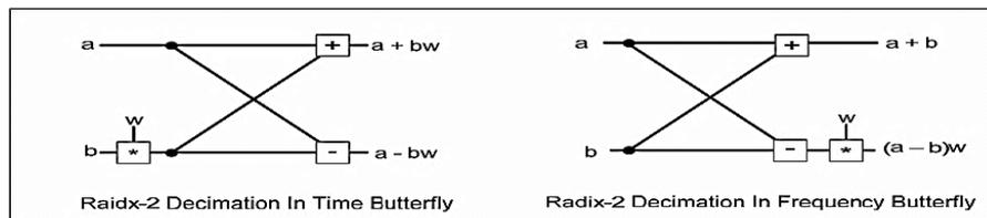
Figure 1: Radix -2 Butterfly Structure
