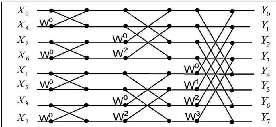
Figure 3: 8-Point Radix -2 DIF FFT Using Butterfly Structure
