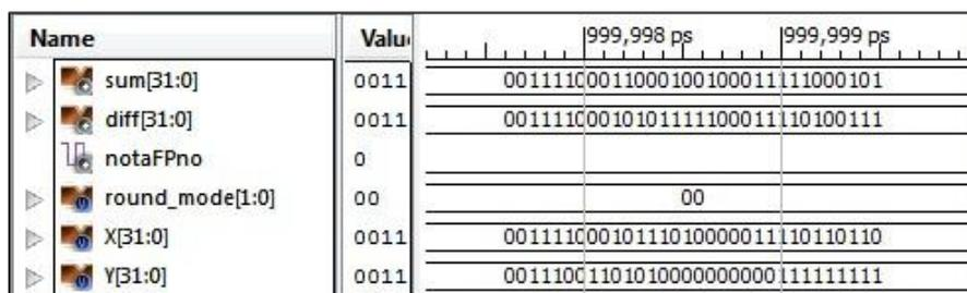
Figure 5: Timing Simulation waveform of Proposed FFPAS module
