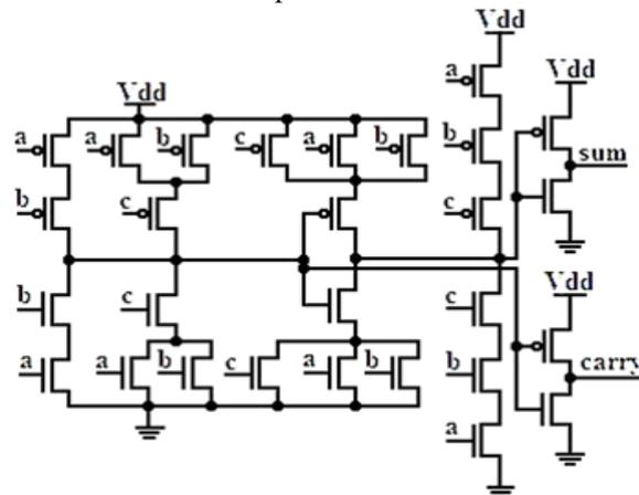
Figure 4: Circuit design of 28T full adder design (CMOS design style).
