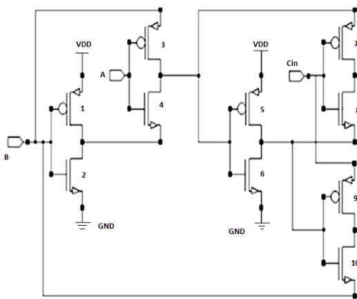
Figure 3: Circuit diagram of 10T GDI design style
