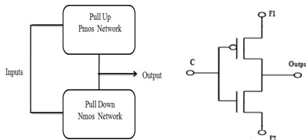
Figure 1. Pictorial representation of (a) CMOS design style and (b) GDI design Style
