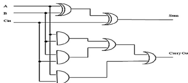
Figure 5: Circuit diagram of 54T full adder design
