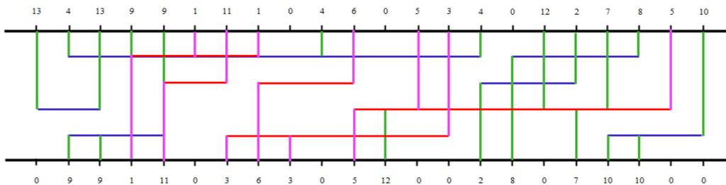
Fig.4. Routing Solution using Four Layers
