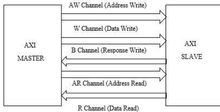
Fig. 1. Block diagram of AMBA AXI
